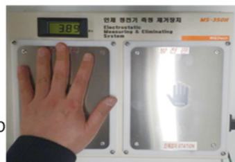
• Measured value of human static electricity detected from the detecting plate: 3.89kV
