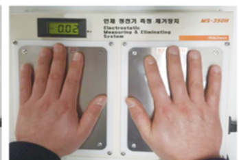
• Measured value of human static electricity detected from the discharging plate: 0.02kV
