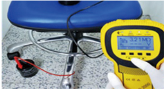
Measuring the energization resistance of antistatic chair and antistatic tile
