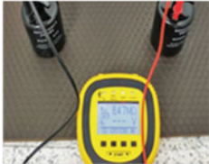
Measuring the resistance of surface of the antistatic mats
